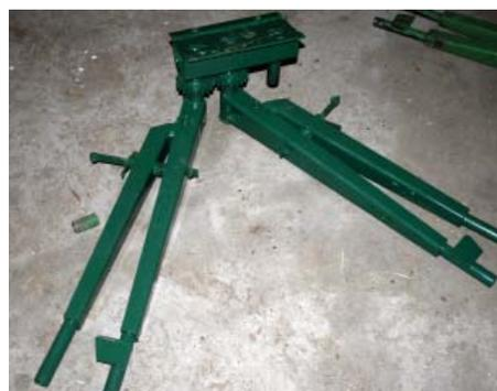
Qwicktie twine arms are designed to replace the existing twine arm hardware on Deere and New Holland big round balers (above). The fast twine tie system uses four arms, providing a covering that's nearly equal to netting for rain and weather protection.
