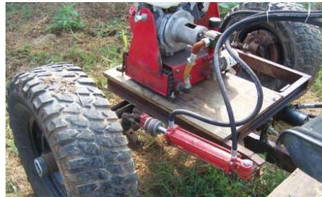
Neal Grose "self-propelled" his tow-behind wrapper, fitting the front end with the front axle off a 1981 4-WD truck (above). A 10 hp hydraulic power unit from a post hole auger provides power, and a salvaged hydraulic motor attaches to the front axle differential to drive the rig.
