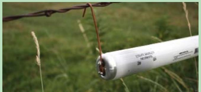
Elroy Lindaas hangs a burned-out, 4-ft. long, 40-watt fluorescent bulb on electric fence. Bulb lights up with each surge of fence charger.
