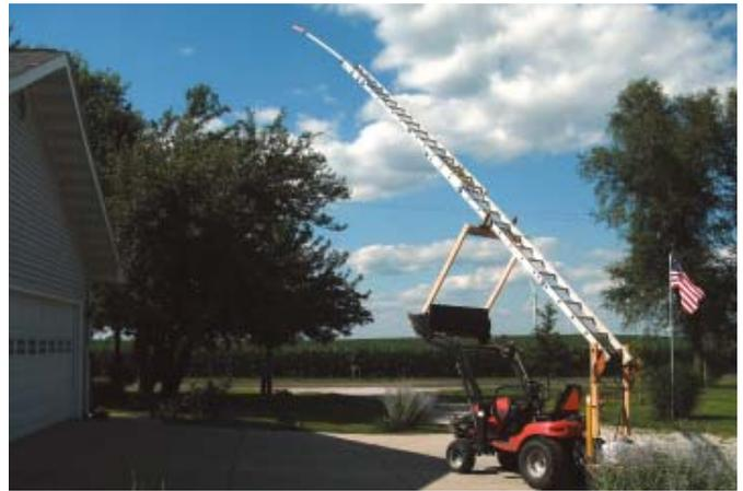
To spray the tops of his apple and elm trees, Ron VanEtten lifts a 32-ft. aluminum extension ladder high over his 20 hp compact tractor. A 10-ft. long homemade spray boom attaches to top of ladder.
