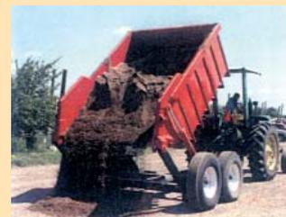
The NTH MX-8 “high lift” dump trailer rides on tandem walking beam axles and has a capacity of 8 tons (above). The box raises straight up and dumps out the back like a dump truck, allowing you to make piles up to 4 1/2 ft. high with no hand unloading (above right). With the tailgate lowered to the ground, the rig can be used to haul a skid loader down the road to the next job.
