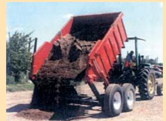
The NTH MX-8 “high lift” dump trailer rides on tandem walking beam axles and has a capacity of 8 tons (above). The box raises straight up and dumps out the back like a dump truck, allowing you to make piles up to 4 1/2 ft. high with no hand unloading (above right). With the tailgate lowered to the ground, the rig can be used to haul a skid loader down the road to the next job.
