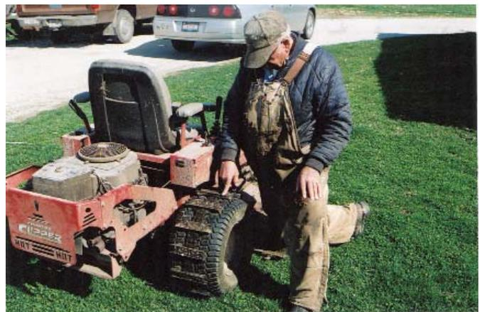
To improve traction on his zero turn riding mower, Roger Foster attached home-built channel iron tracks to the drive tires.
