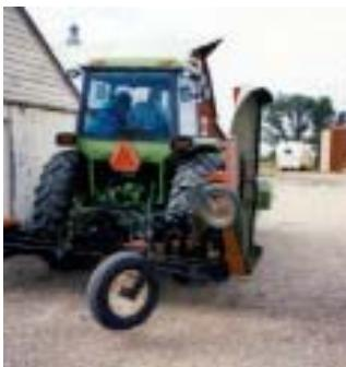
**A 24-in. stroke hydraulic cylinder mounted between an inner frame and the mower deck provides at least 135 degrees of tilt.**
