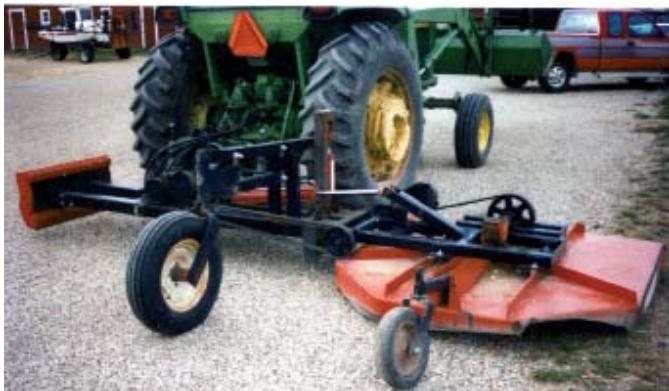
**With its unusual sidearm design, Don Sawvell's mower can go from horizontal to plus or minus 45 degrees without even slowing down.**
