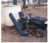
Mark Jenkins modified his Murray 20 hp garden tractor, installing an old Snapper bagger discharge elbow on the 52-in. deck and adding a 300-gal. poly tank on back.
