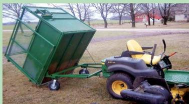
Gerald Auten built this tow-behind trailer to collect grass and leaves behind his Deere riding mower. Trailer's rear door swings to the side for dumping.
