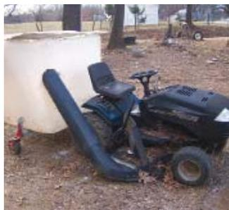
Mark Jenkins modified his Murray 20 hp garden tractor, installing an old Snapper bagger discharge elbow on the 52-in. deck and adding a 300-gal. poly tank on back.
