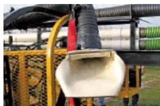
Pickers drop apples into a vacuum tube (left). Rotating foam rubber wheel at bottom of tube catches apples and rolls them onto a distribution disk with canvas blades (right). From there apples roll gently into a bin.
