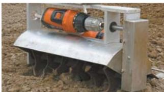
It then doubles back slightly and through a hole in the housing above the drill. From there it extends up to the handlebars. Pulling on the rope tightens the trigger, engaging the drive. To stop the tiller, all Coleman has to do is release the tension on the rope.
