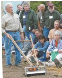
Eliot Coleman’s garden tiller is powered by a battery-operated electric drill.
