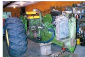
The head is off an LP-powered Deere 60.
