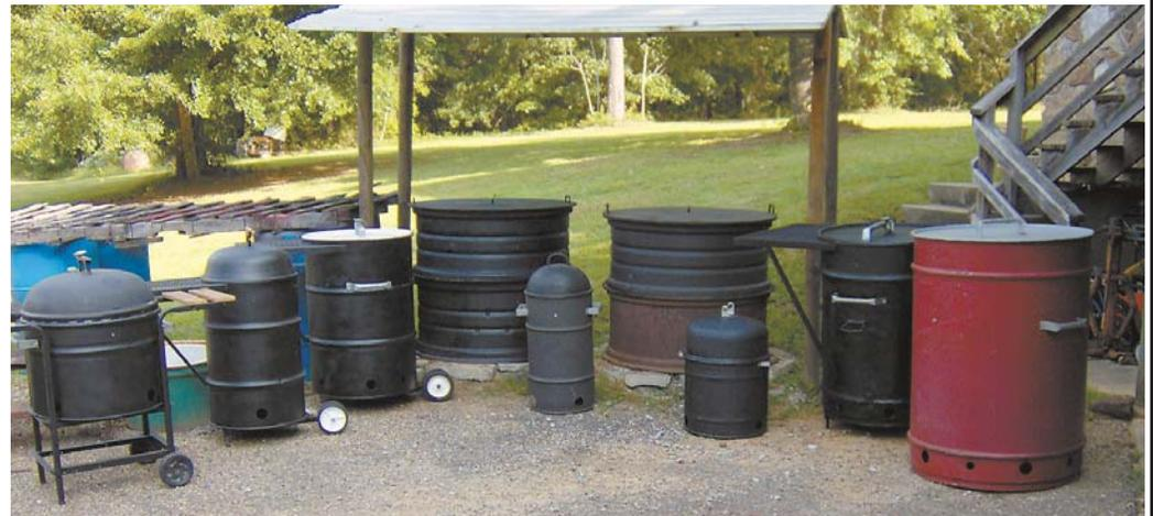
Major Dunlap has a thriving sideline business selling barbeque grills made out of scrap materials. The fire is cradled by a high carbon steel harrow disc, which rests on a 3-legged tripod inside each drum. He uses 10, 15, 30, 85 and 110-gal. drums.
