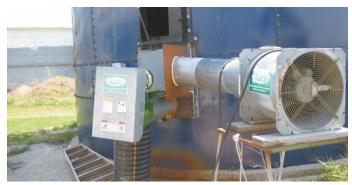
Walt and Gerry Ackermann converted an old Harvestore into a 7,000-bu. storage bin with air-drying capability. Photo shows new entry door with auger and air plenum.
