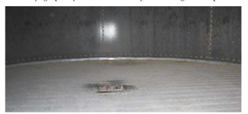
A 5 hp, 20-in. fan pulls air down through drying floor in the 20 by 32-ft. structure.
