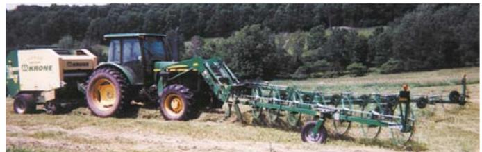
Wivell modified a Frontier V-wheel rake to fit the front-end loader on his Deere tractor. He uses it to rake to the center of tractor, pulling a Krone round baler behind.
