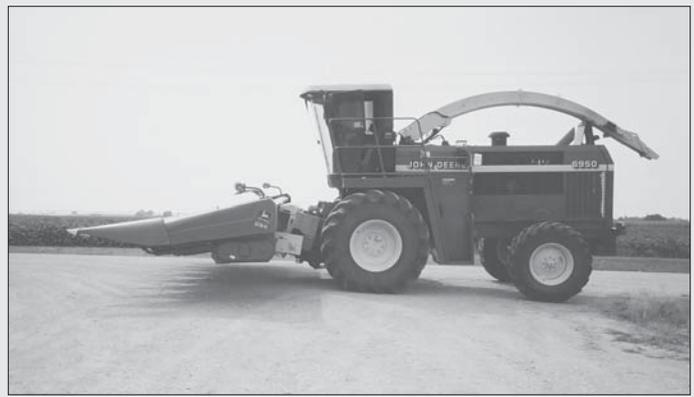
Adapter plate lets you use a corn head on a self-propelled forage chopper, turning it into an ear corn only chopper. Adapters are available to fit several brands.
