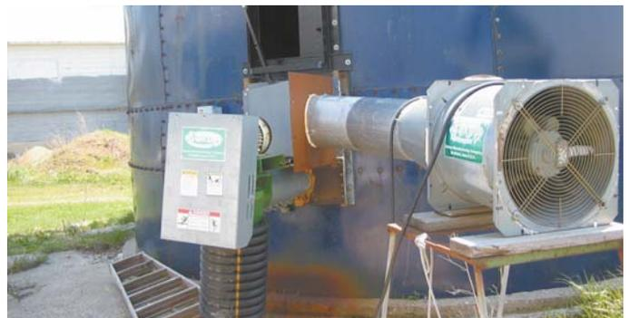
Walt and Gerry Ackermann converted an old Harvestore into a 7,000-bu. storage bin with air-drying capability. Photo shows new entry door with auger and air plenum.
