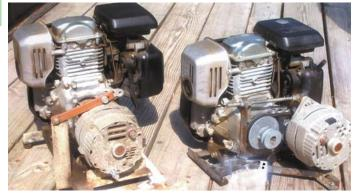
Generator at left direct-drives alternator. Genset at right has a belt drive.
