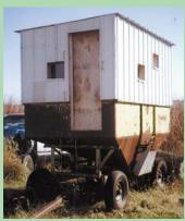
Max Dunlap used 2 by 4's, sheet metal, and plywood to make this portable deer stand on an old gravity flow wagon.
