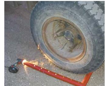
A flashlight can be stuck into end of L-shaped pipe at night for good visibility.
