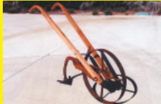
My father, Nat Ashby, made this garden cultivator during WW II when metal was hard to find. I still use this cultivator today. The hub is an old tractor piston - the wrist pin acts as the pivot point. Dad threaded the inside ends of the wrist pin to allow the bolts to support the handles. The rim of the wheel was cut from an old barrel. **(Robert Ashby, Dammeron Valley, Utah)**
