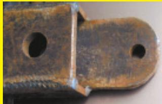
In order to pull wagons out of a field with our big 4-WD tractor, I needed a 1-in. dia. drawbar hole instead of the larger 1 1/2-in. hole in the 4-WD's drawbar. So I welded together an add-on hitch that slips over the drawbar and pins in place with a 1 1/2-in. pin. Then the wagons can be hitched to the smaller hole. Simple and it works. **(Jason Engel, Tiskilwa, Ill.)**
