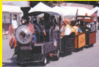
car aluminum mounted on a metal frame-work. The single-axle cars ride on dual wheels and are made from 1-in. angle iron and race car aluminum. One of the trains can haul 24 kids at a time.
