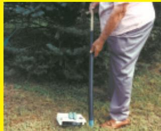
Just drop the spike down the pipe and drive it into the ground by pounding on the wood handle with a hammer. The spikes should be driven 2 in. below the surface, which is easy to do with this setup. **(C.F. Marley, Nokomis, Ill.)**
