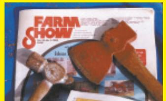
To hold hammer and ax heads in place I drill a small hole through the center of the head, then place a nail through the hole and cut it off about 1/8 in. on the opposite side. Then I place the nail head on a vise or anvil and use a ball peen hammer to flatten the end of the nail like a rivet. **(Leonard Seltzer, 16040 W. Elmwood, Manhattan, Ill. 60442 ph 815 478-3578)**
