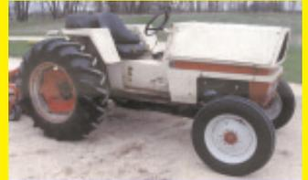
I redesigned the tractor to my liking and have used it around my farm for all these years. I also replaced the original 20 hp, 2-cyl. air-cooled engine with a 30 hp, 4-cyl. water-cooled model. I replaced the original hydrostatic transmission with a 3-speed transmission. I had to move the gas tank, originally located in front of the engine, behind the operator in order to make room for the radiator. The hood was then modified to make room for the radiator.
