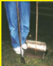
which extends below the floor of the pan, opens the lid when the scooper is in the lowered position - thanks to a small piece of angle iron attached to the pan handle. When you lift it back up, the bottom swings down so the doo-doo drops to the back of the pan. I duct taped a putty knife to a broom handle to push poop into the pan. **(Rex Gogerty, Hubbard, Iowa)**
