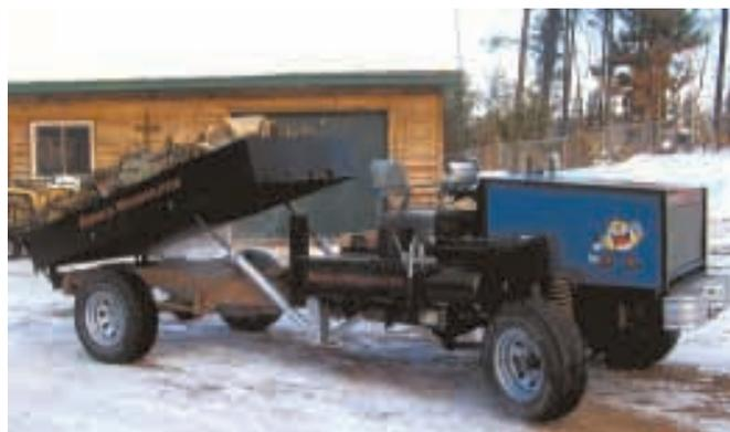
Converted pickup has a homemade log splitter on one side and a dump box on back.
