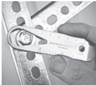
**V-shaped opening at one end of tool has a variable pitch tooth design, allowing tool to grip almost anything.**
