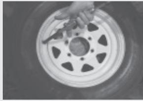
and blow-off gun with the safety tip removed, allowing a larger volume of air to enter the tire. When the tire seats on the rim the valve core can be replaced, and then the tire is aired up normally."
