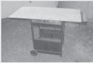
**Matt Studer, New Washington, Ohio:** "Have you ever wondered what to do with that old gas grill that has rusted out? Instead of taking it to the landfill or turning it into scrap iron, why not make yourself a rolling tool cart. That's what I did. I removed the grill section and screwed a 24 by 36-in. piece of plywood to the frame. It works great around the shop, holding tools or parts wherever I'm working."
