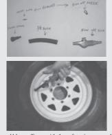
and blow-off gun with the safety tip removed, allowing a larger volume of air to enter the tire. When the tire seats on the rim the valve core can be replaced, and then the tire is aired up normally."
