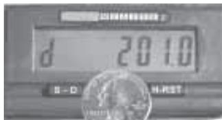
**FastMeasure system can be installed on anything that rolls. Display shows distance in feet or meters and speeds in feet per minute, mph or kilometers per hour.**
