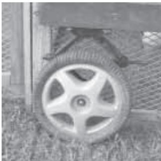
A screw-type jack, mounted upside down, attaches to each wheel. Greise cut a pin off the top part of jack and then bolted on the wheel's original bracket and axle.
