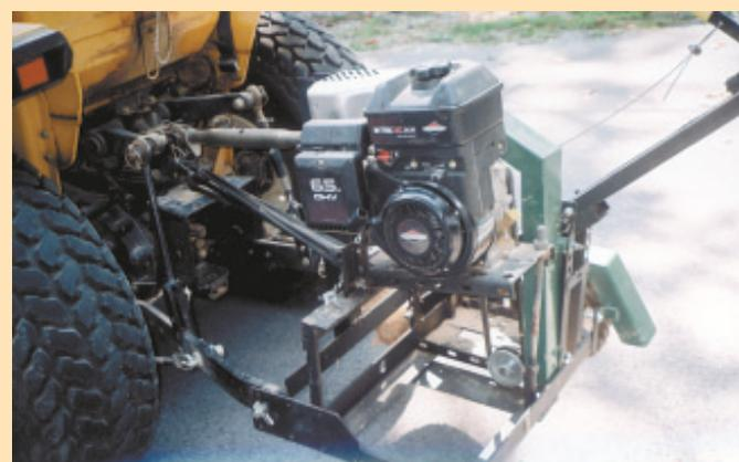
Stump grinder swings up to 12 in. from side to side across the stump. Flexibility is provided by loosening sway chains on 3-pt.'s lower lift arms.
