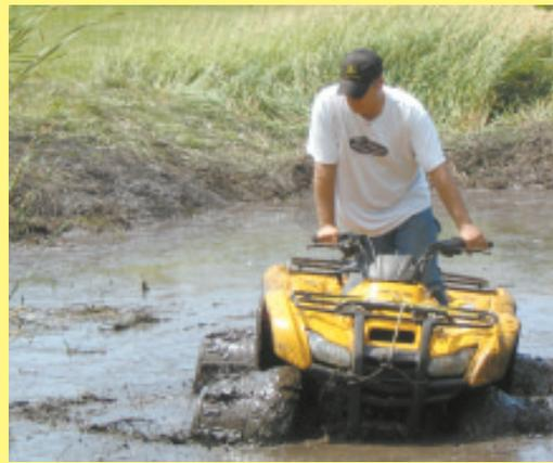
J-wheelz hubs bolt onto ATV's existing wheels, widening them in a way that helps in deep mud without affecting the road drivability.
