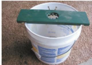
Six wood dowels protrude into ear corn-sized opening. As cob is twisted against dowels, kernels fall into bucket.
