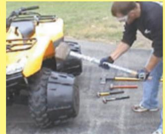
Replaceable rubberized traction blades fit into slots on hubs.
