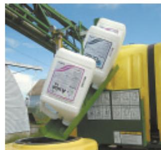
Stand consists of a 25-in. long, V-shaped trough fitted with four evenly spaced rods.
