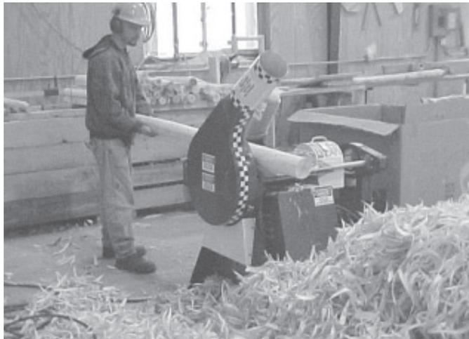
**German-style log peeler removes bark from logs that are used for railing, furniture and log home construction.**
