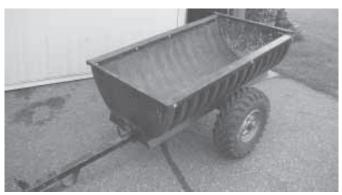
Dump cart is made out of a 5-ft. section of 32-in. dia. culvert cut in half lengthwise.
