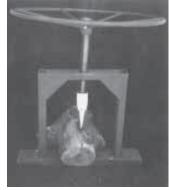
Large diameter metal wheel works like a drill press to split logs.
