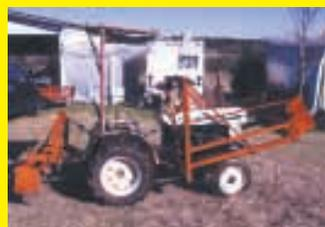
Here's a photo of a high-lift mini loader that I built for my garden tractor using plans from Larry Walton (Vol. 32, No. 3). I beefed up the frame with bigger tubing and made the bucket out of a used barbecue grill.
