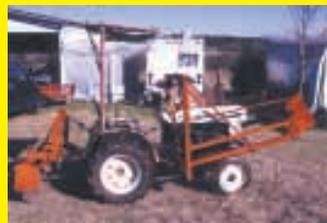
Here's a photo of a high-lift mini loader that I built for my garden tractor using plans from Larry Walton (Vol. 32, No. 3). I beefed up the frame with bigger tubing and made the bucket out of a used barbecue grill.
