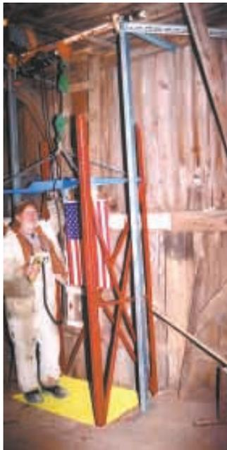
**Gene Boehler needed a way to take big parts and other items up to the loft storage area in his shop, so he built this elevator. It can lift up to 900 lbs. and rides up through an existing opening in the hayloft floor.**
