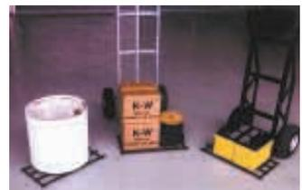
**A pair of 1/2-in. sq. support tubes on outside edges of pallet keep the load 1/2 in. off the floor, allowing you to easily slide a hand truck under the load.**
