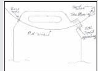
**R. E. Dickinson, Theodore, Alabama:** "My neighbor came up with this vent for plastic fuel cans. After draining and drying the inside of the can, drill a hole in location as per the drawing using a 1/2-in. drill bit. Invert the can and shake out any drill cuttings (that's why you need a dry can). Push a 3-ft. length of wire through the drilled hole and then out the filler spout hole.
