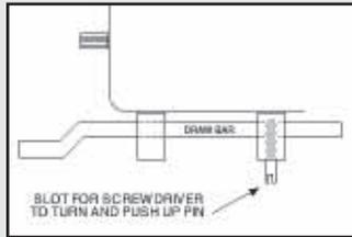
**David P. Campbell, Elnora, Ind.:** "I ground a slot in the bottom of the drawbar pins on my Deere 4020 and 2520 tractors. Makes it easy to use a screwdriver to turn and push up on the pin when you need to lengthen or shorten the drawbar as needed for whatever job you're doing."
