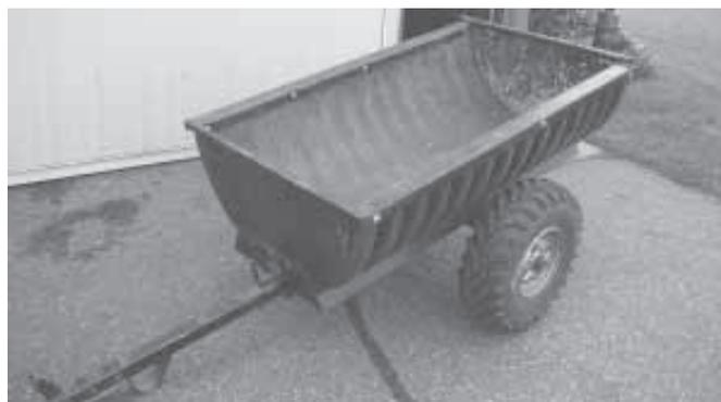
Dump cart is made out of a 5-ft. section of 32-in. dia. culvert cut in half lengthwise.
