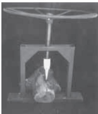
Large diameter metal wheel works like a drill press to split logs.
