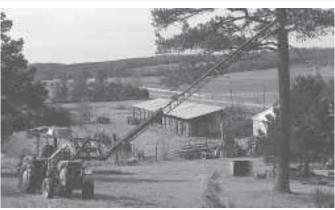
Loader-mounted 30-ft. TV antenna has an electric chainsaw on one end. A pto-driven generator on back of tractor powers the saw.
