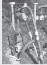
Hanger keeps Dwayne Oxford's 3-pt. mounted post-hole auger off the ground so it's easy to hook up to a tractor.
