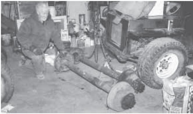
Instead of buying new axles for a couple trailers they were building, Clair Wilson and sons modified axles off Ford 3/4-ton and 1-ton pickups.
