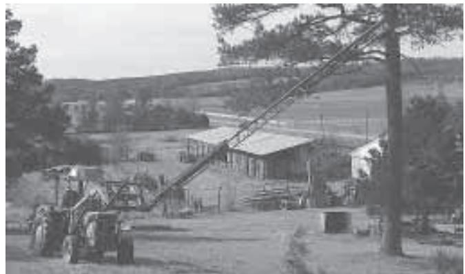
Loader-mounted 30-ft. TV antenna has an electric chainsaw on one end. A pto-driven generator on back of tractor powers the saw.
