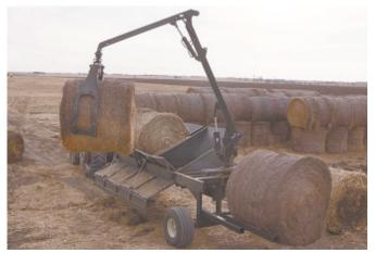
Two-bale processor uses a grapple to load bales. It can feed out two bales at once, blending different types of forage.
