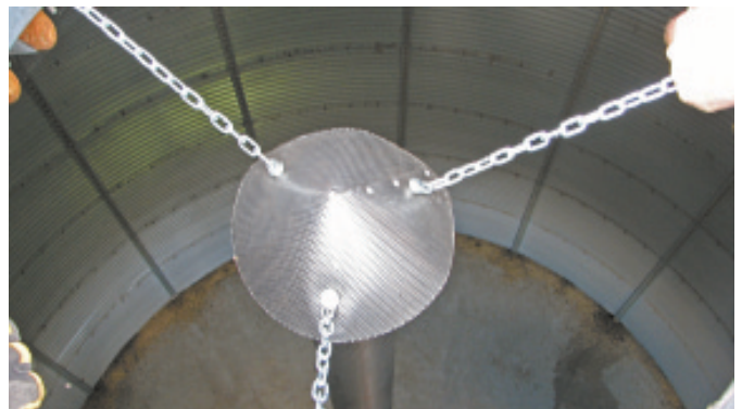
Vertical, 6-in. dia. perforated pipe installs up the center of bin to cool, dry and ventilate grain. Eliminates the need to use fans or outside energy.
