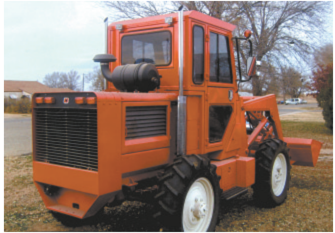
Engine is a Chevy 350 equipped with a Power-Glide transmission.
