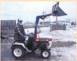
Russell Wright converted an old Roper garden tractor into a dandy loader tractor. A beltdriven hydraulic pump on one side of tractor is used to raise and lower the bucket and also to tilt it.
