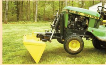
George Liskey converted a Deere model 43 front blade into this "bucket loader". Bucket's bottom and sides were made by welding 3/8-in. thick steel plate onto blade. Deere 332 16 hp diesel tractor and built an turer. He expects the unit could be sold for
