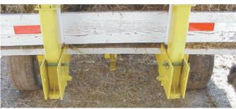
Hundertmark used parts from an old bean bar to build rack's hinge system.
