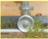
Removeable rubber wheels can be attached to the skid plates, or units can be set up on permanent pipe tracks with fixed steel rollers.
