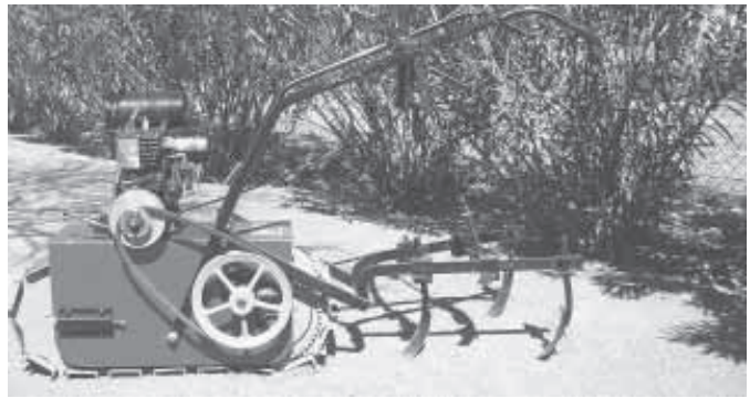
A “crawler-type cultivator”, the Gray Gardener runs on a 7 1/2-in. wide single track.
