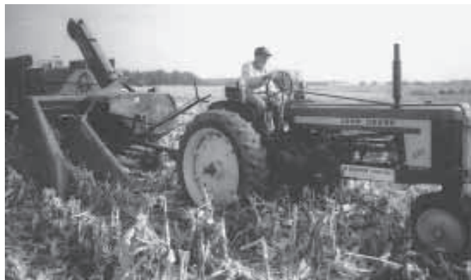
Last fall Ed used the Deere 520 tractor to pull a No. 18 Deere corn picker. Photo was taken just after he had harvested an acre of ear corn.
