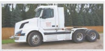
On-the-go tire inflation system lets truck drivers deflate tires as low as 30 psi for better traction in sand or mud, and then inflate them back up for highway travel.
