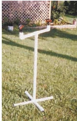
**Pair of rotating sprinklers on top of 4-ft. high pvc frame fling water out in two 45-ft. dia. circles. The sprinklers can be set to rotate in opposite directions.**
