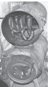
Stove was made from a 30-gal. water pressure tank mounted on four pipe legs. An old 20-gal. oil barrel that serves as the smoker is bolted on top of stove. Homemade sausages hang from metal rods.
