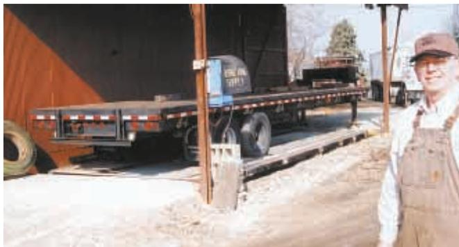
Mark Musser used the bed from a 35-ft. semi trailer as the platform for his home-built weigh scale. He installed four load cells under it, one at each corner.
