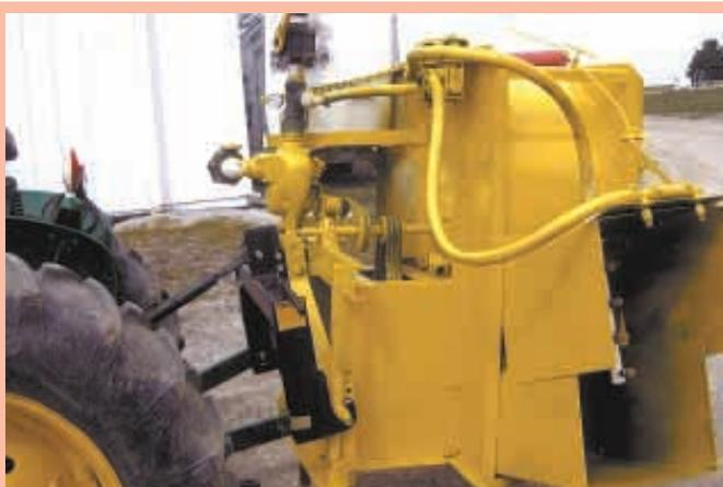
Tractor pto belt-drives a big 28-in. dia. squirrel cage fan and a spray pump.
