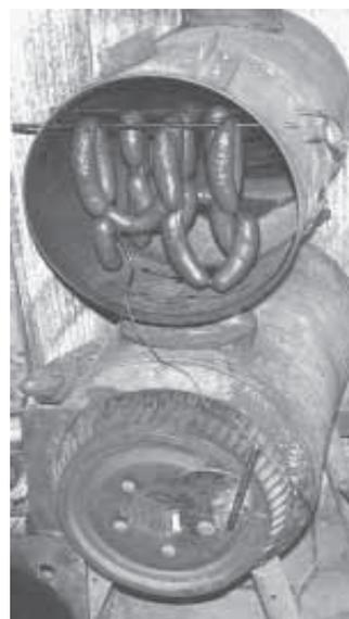
Stove was made from a 30-gal. water pressure tank mounted on four pipe legs. An old 20-gal. oil barrel that serves as the smoker is bolted on top of stove. Homemade sausages hang from metal rods.
