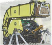
Bale holder attaches to back part of baler and extends up and over top of machine. It collects and holds up to seven bales.
