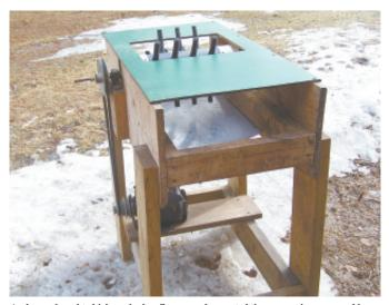
Anderson bought chicken plucker fingers and mounted them on a pipe, powered by an electric motor
