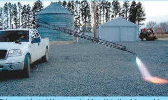
Pickup-mounted, extendable arm moves torch from side to side and also up and down.
