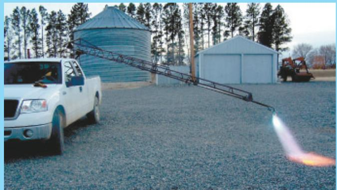
Pickup-mounted, extendable arm moves torch from side to side and also up and down.
