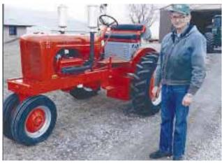
The Litchfields fitted an old Allis Chalmers WC tractor with a Chevrolet 283 V-6 engine and mounted a Mig welder under an extra wide seat.
