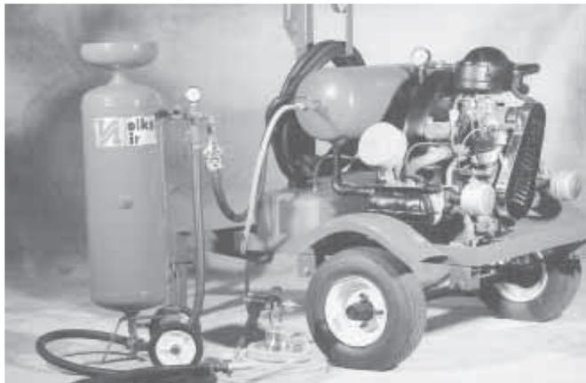
Air compressor kit turns VW engine into high capacity sandblaster.
