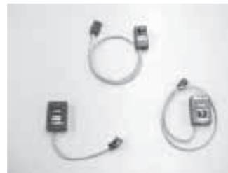
Service kit hooks up to planter sensors and allows Steidinger to simulate ground speed in his shop.
